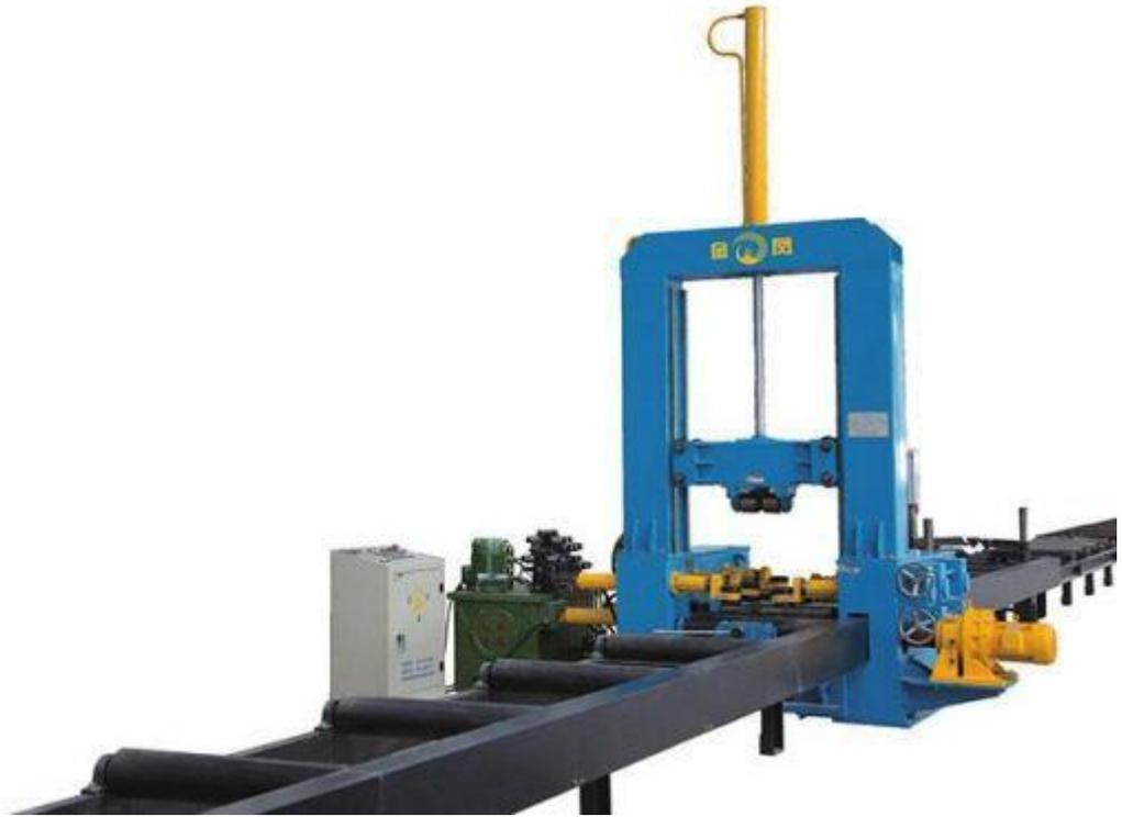
**HG H beam assembling machine**
